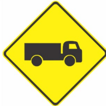
FIGURE 6.1: Typical W5-22 Sign Face (TfNSW)
